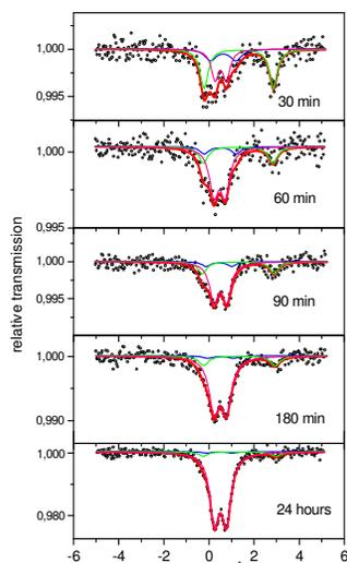
Mössbauer spectra of iron deficient cucumber roots supplied with 0.5 mmol <sup>57</sup>Fe-citrate for 0.5, 1, 1.5, 3, 24 hours. (red line)
