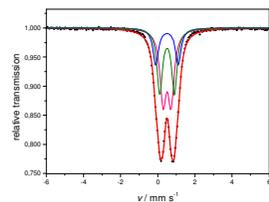
Mössbauer spectra of iron sufficient cucumber roots supplied with 10 μM <sup>57</sup>Fe-citrate for the 3-week growth period. (red line)
